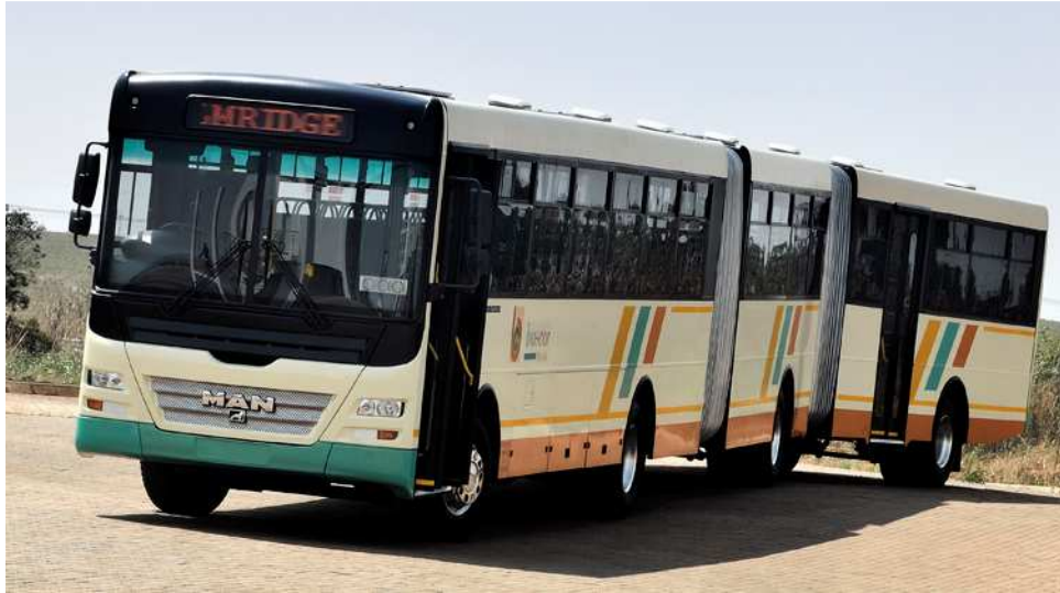
Figure 6 Bi-articulated bus manufactured by MAN Bus & Coach
