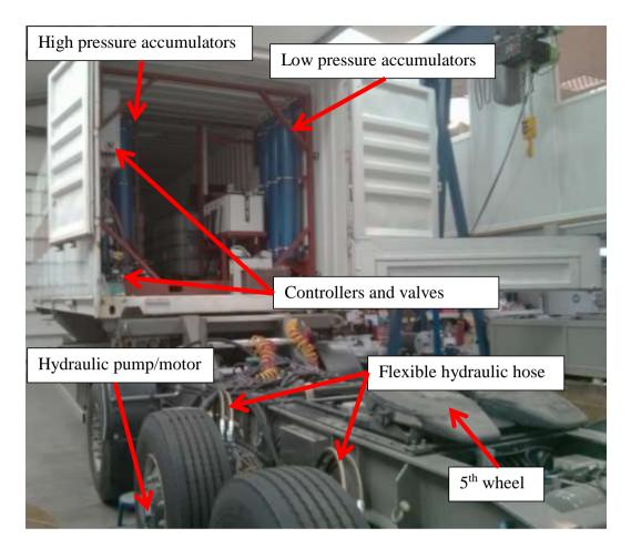
Figure 7 – Assembled regenerative braking trailer
