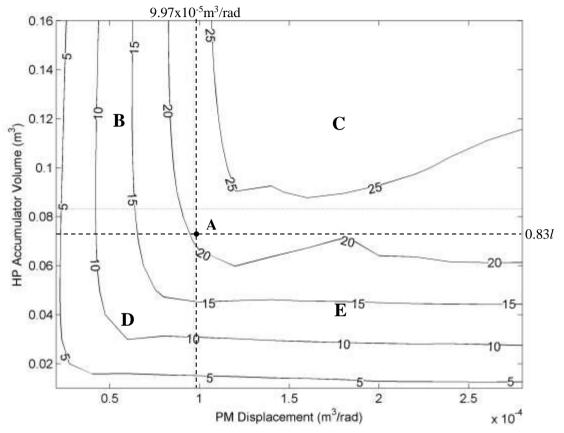
Figure 4 – The reduction in EI<sub>v</sub> (%) achieved by regenerative braking over a 700m, 30mph (13.41m/s) stop-start cycle. The selected design is at point 'A'.
