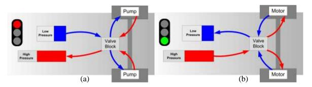
Figure 1 – Hydraulic regenerative braking system schematic showing system in (a) deceleration and (b) acceleration (arrows show fluid flow)
