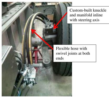
Figure 8 – Close-up showing the pipe routing on the rear axle which enables  $\pm 30^{\circ}$  of wheel steering and full suspension travel without stretching or twisting the hydraulic hoses
