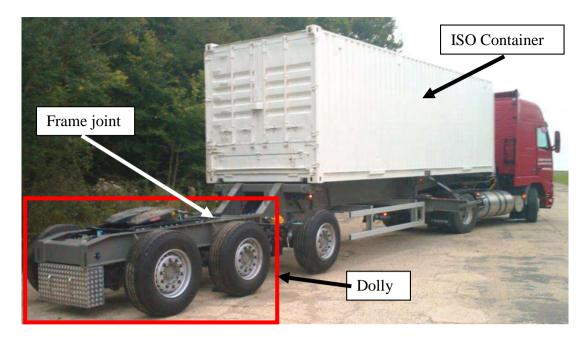
Figure 9 – CVDC test B-link trailer before modification. Highlighted axles are steerable and were used for the experimental system
