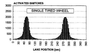
Figure 4. Pattern of single tired wheels
