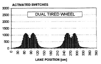
Figure 5. Pattern of dual tired wheels
