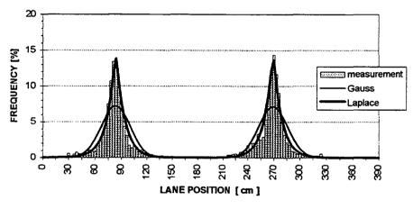
Figure 8. Theoretical wheel path distribution
