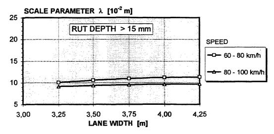
Figure 11 Correlation between scale parameter  $\lambda$  of lateral shift, lane width and speed for a road section with heavy rutting
