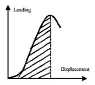
Figure 2. The curve of impact tenacity.
