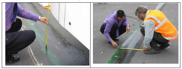
Figure 2. Tail swing measurement.
