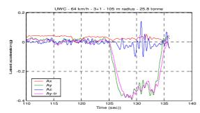
Figure 9: Acceleration versus time– 105 m radius curve – UWC 3+1
