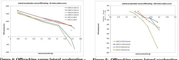
Figure 4: Offtracking versus lateral acceleration – 35 metre radius curve Figure 5: Offtracking versus lateral acceleration – 105 metre radius curve
