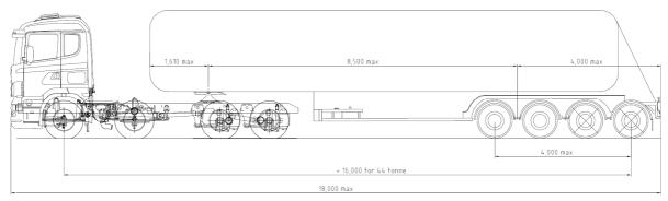
Figure 1: 8x4 tractor unit and quad-axle semi-trailer with two rear self-steering axles
