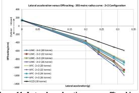
Figure 11: Lateral acceleration versus offtracking – 2+2 quad configuration, UWC and APC
