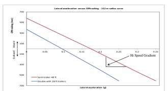
Figure 3: Offtracking - tractor semi-trailer and double combination - 152 m radius curve, source (Ervin and Guy 1986 - p.33)
