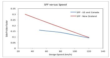
Figure 2: Design Side Friction Factor versus Speed – North America and New Zealand
