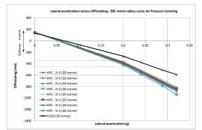
Figure 13: Lateral acceleration versus offtracking – 2+2 and 3+1 quad configuration- APC
