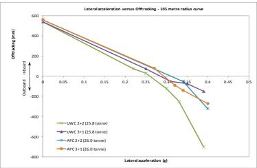
Figure 15: Offtracking versus lateral acceleration – 105 m radius curve – with creep speed results added
