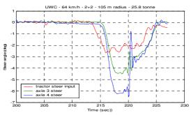
Figure 8: Tractor steer input, trailer axle 3 and 4 steer – 105 m radius curve – UWC 2+2
