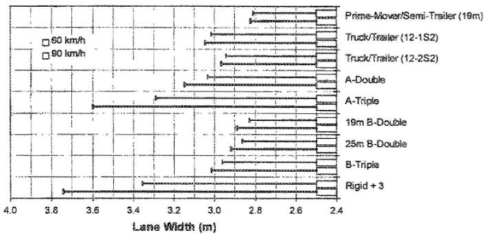
Fig. 10 Estimated lane width requirements for a range of heavy vehicles.
