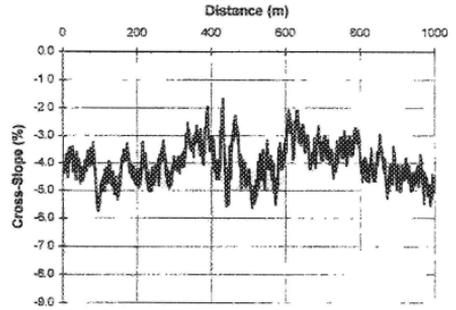
Fig. 4(b) Cross-slope profile measured on Test Section C.
