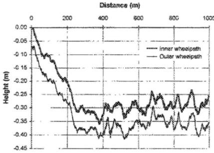
Fig. 4(a) Wheelpath profiles measured on Test Section C.
