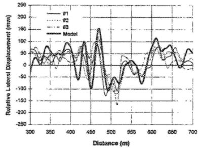
Fig. 8(b) Comparison of measured with predicted over 300 to 700m interval on Test Section C at 75 km/h.
