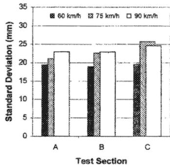
Fig. 6 Prime-mover lateral displacement from the accelerometer-based system.
