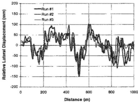
Fig. 2 Lateral displacement from the video-based system - 60km/h on Test Section C.
