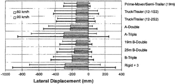
Fig. 9 Bar and whisker plot showing lateral displacement of rear trailer ( $\mu \pm 3\sigma$ ). The hauling unit is located at the origin (zero).
