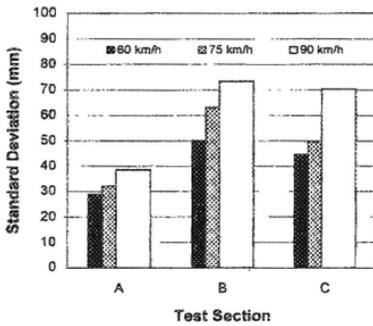
Fig. 5 Relative lateral displacement of rear unit from video system on the A-Double.
