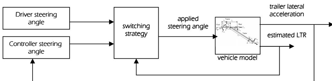
**Figure 9** – Steering control loop
