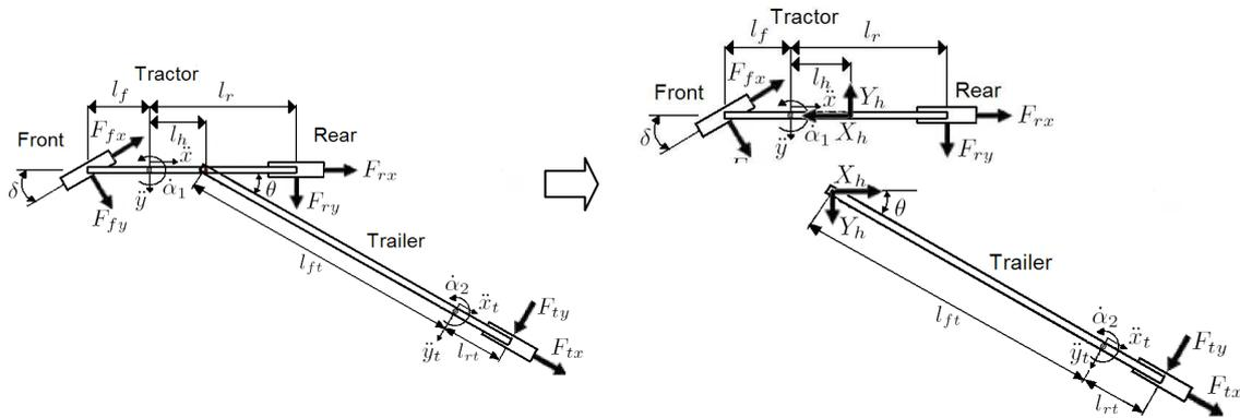
**Figure 1** - Extended semi-trailer bicycle model
