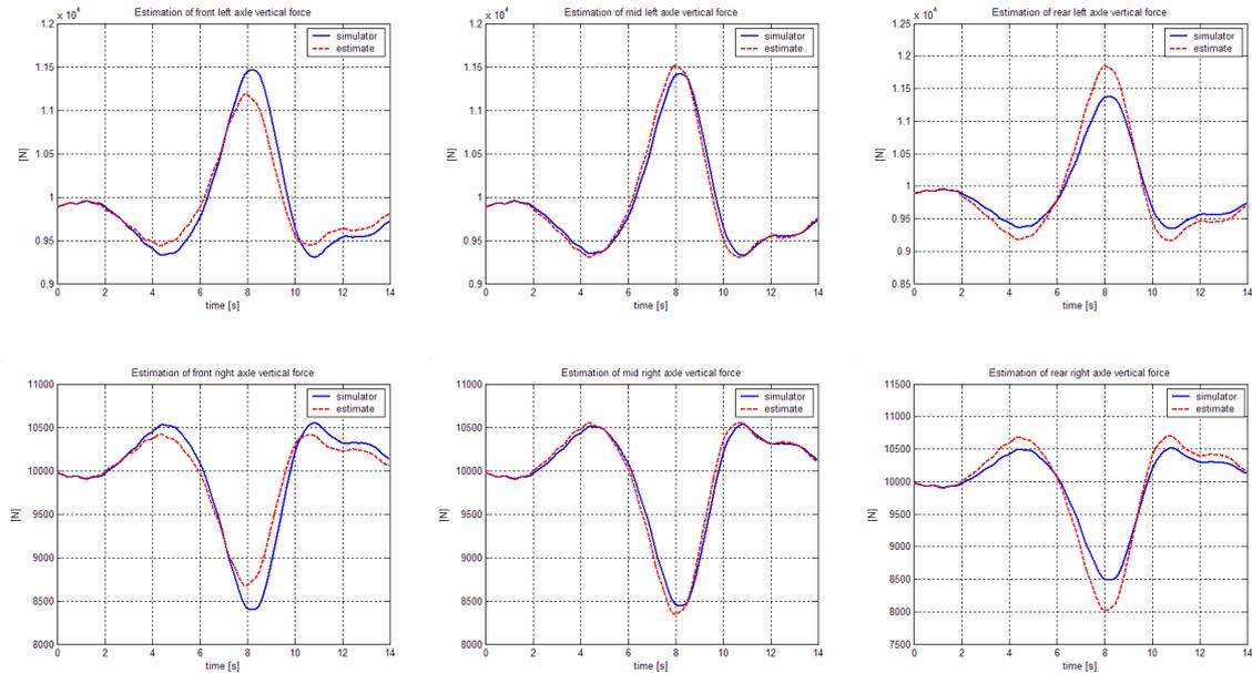
**Figure 7** - Estimation of trailer vertical forces (from left to right: front, mid and rear trailer axle; up to down: left and right wheels) using adaptive observer method
