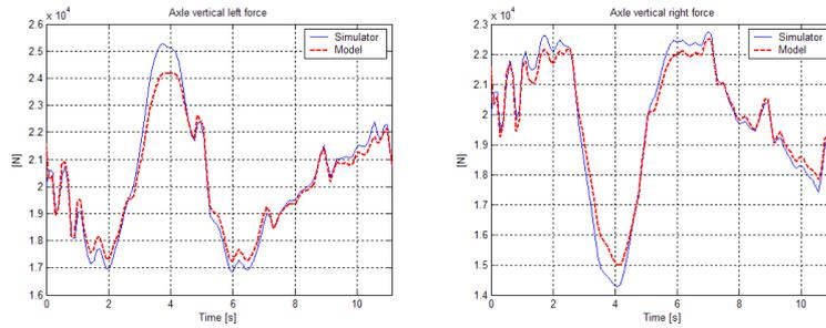
**Figure 5** - Simulator (solid) and model (dashed) axle vertical forces for double lane maneuver
