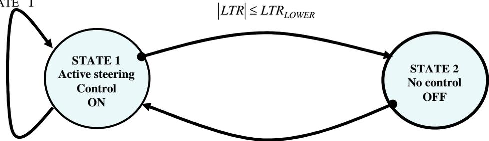
**Figure 8** – Hybrid control scheme
