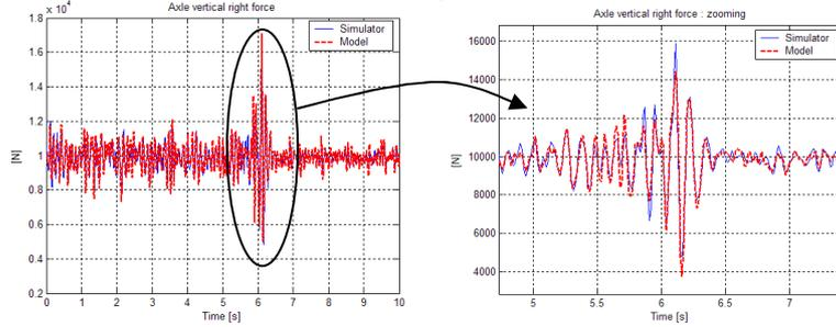
**Figure 4** - Simulator (solid) and model (dashed) axle vertical forces for straight line maneuver
