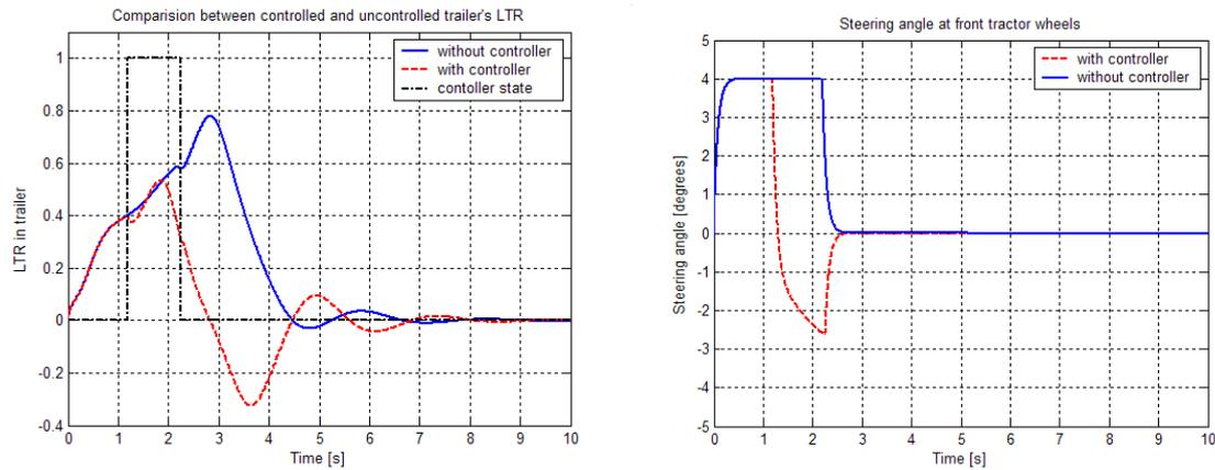
**Figure 10** – Left: the total LTR in the trailer with and without controller, right: the steering angle with and without controller
