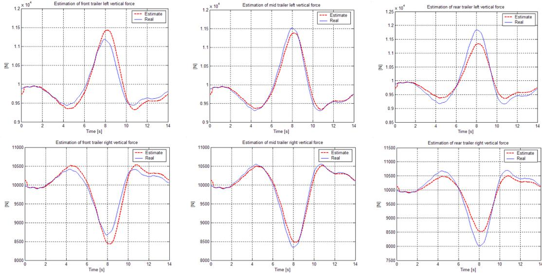
**Figure 6** - Estimation of trailer vertical force (from left to right: front, mid and rear trailer axle; up to down: left and right wheels) using inverse model method
