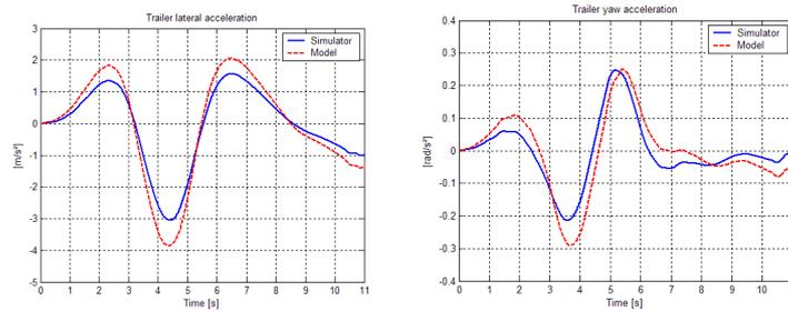
**Figure 3** - Simulator (solid) and model (dashed) trailer accelerations (left: lateral, right: yaw)
