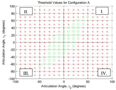
Figure 11. Controllability limits vehicle combination A
