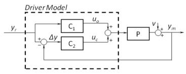
Figure 2. Driver model structure
