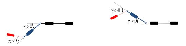
Figure 8. Situations when the second articulation angle is not visible for the driver
