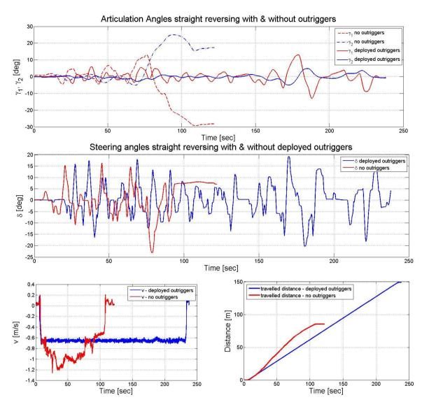
Figure 7. Performance comparison for the driver with and W/O deployed outriggers
