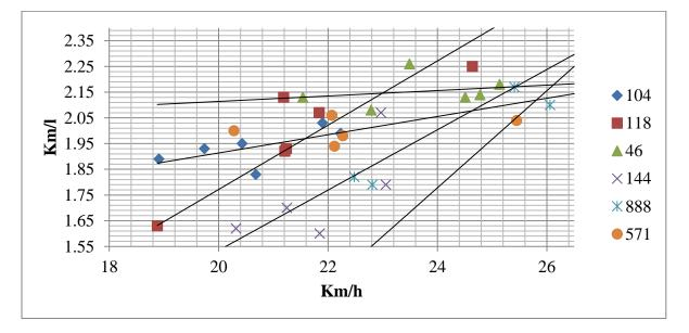
Figure 2. Fuel Consumption as a function of Vehicle Average Speed for 6 Vehicles
