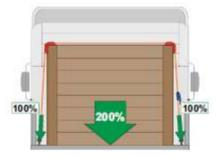
The use of large corner protectors can contribute to the distribution of lashing forces over a greater zone and thus to the reduction of the movement of the cargo.
