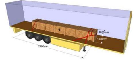
The trailer has an ordinary plyfa floor that is swept clean and is free from frost, ice and snow. The trailer is built in accordance with the EN 12642 standard, XL class, and the lashing points on the trailer are designed in accordance with the EN 12640 standard, each with a lashing capacity (LC) of 2000 daN. The transverse distance between the lashing points is about 2.4 m.
