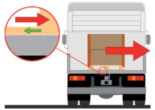
Centrifugal forces are the forces acting on the vehicle and its load at cornering. They tend to push the vehicle and its load to the outside of the turn. The centrifugal force is calculated using the formula below:
