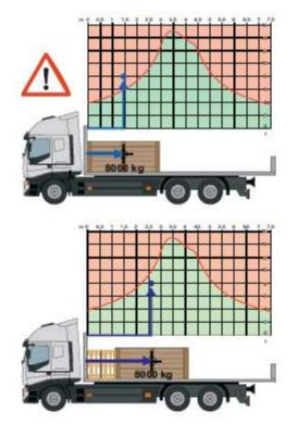
Generally, the maximum pay load may be used only when the centre of gravity is positioned within narrow boundaries about half the length of the loading space.
