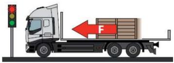
Deceleration forces; when braking, the load tends to slide forward
