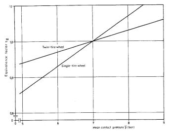
Fig. 8 Equivalence factor for wheel contact pressure
