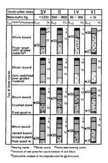
Fig. 1 Standardized structures of bituminous pavements
