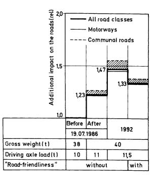
Fig. 13 Additional impacts on the road caused by various vehicle fleets
