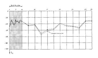
Fig. 9 Measured surface strain on the pavement
