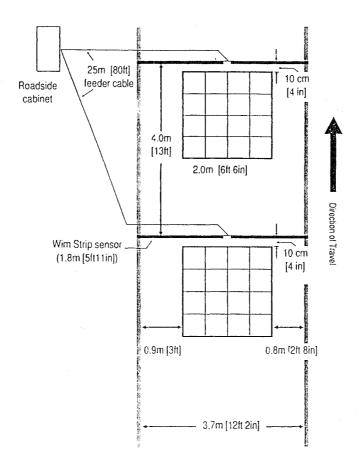
Figure 1. Typical sensor array layout for one traffic lane
