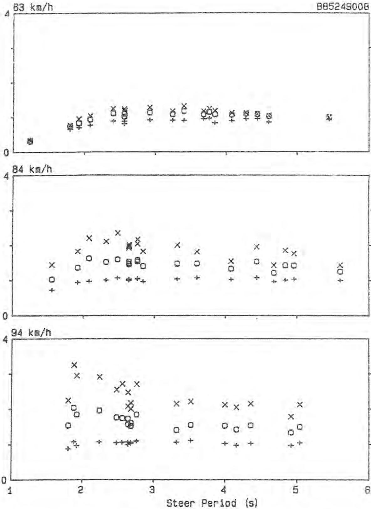
A-train triple, rearward amplification of lateral acceleration
