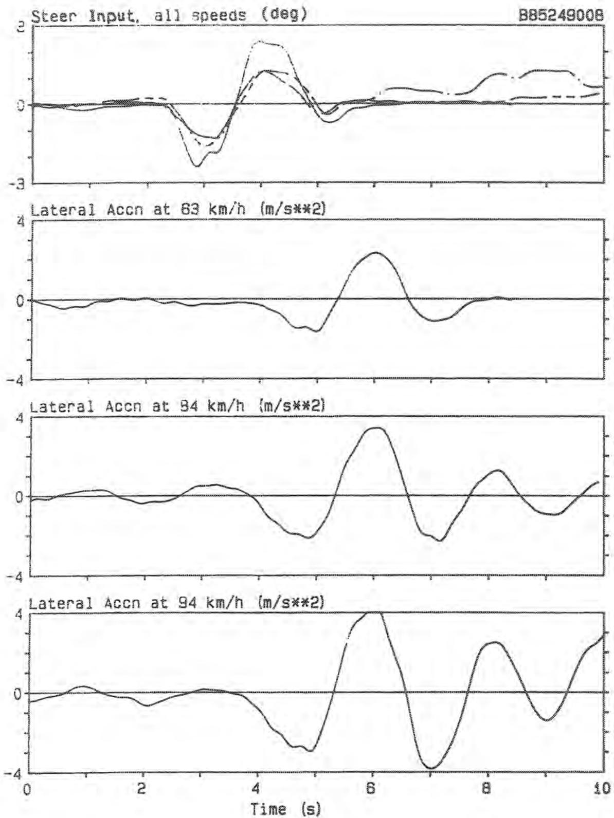
A-train triple, sinusoidal steer, rear trailer lateral acceleration at three speeds
