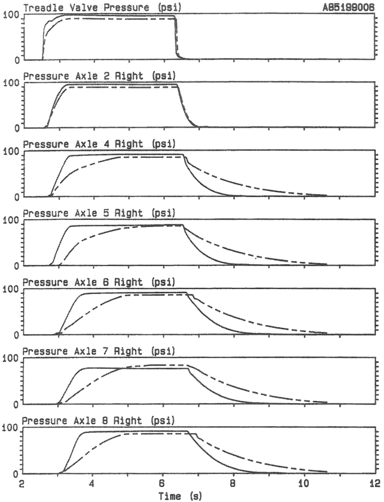
A-train and C-train triples, air brake application and release
