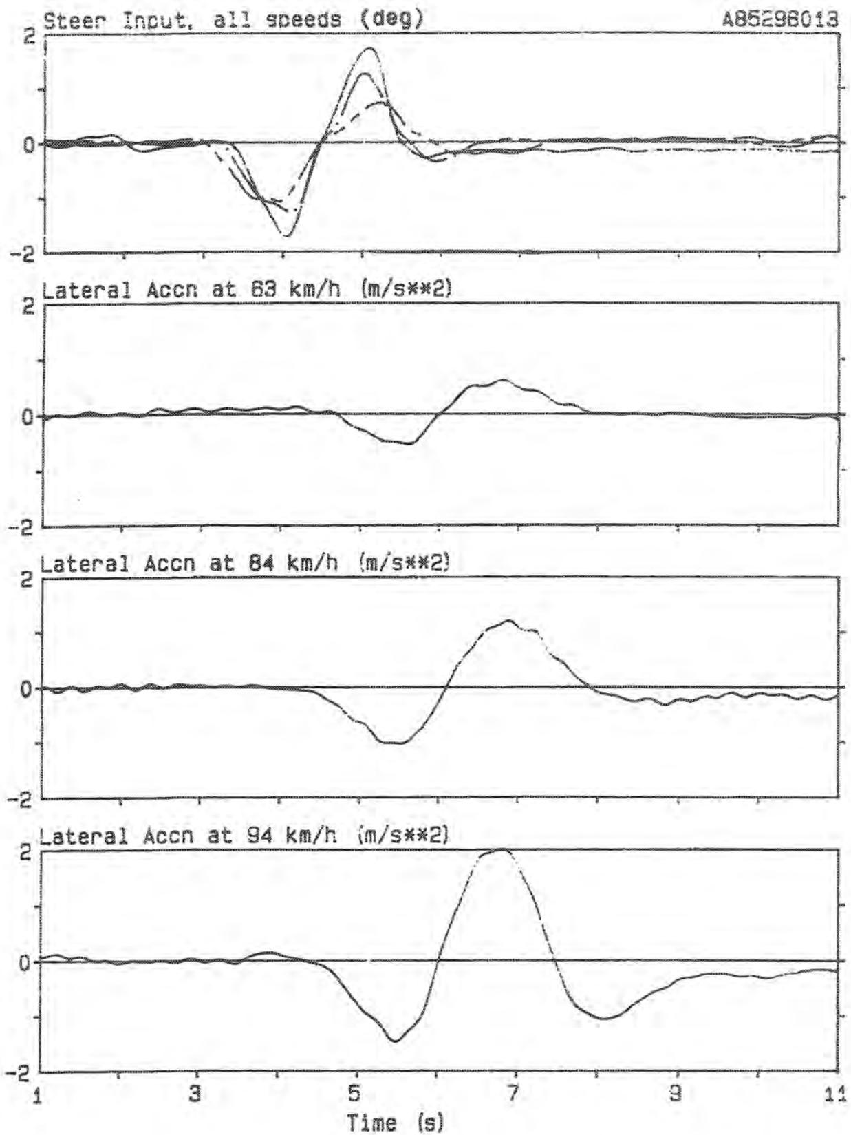
C-train triple, sinusoidal steer, rear trailer lateral acceleration at three speeds
