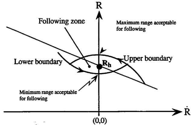
Figure 8. Desired region of operation during following
