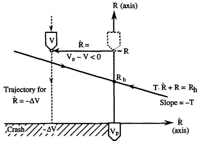
Figure 2. Headway control in the (R-dot, R) space
