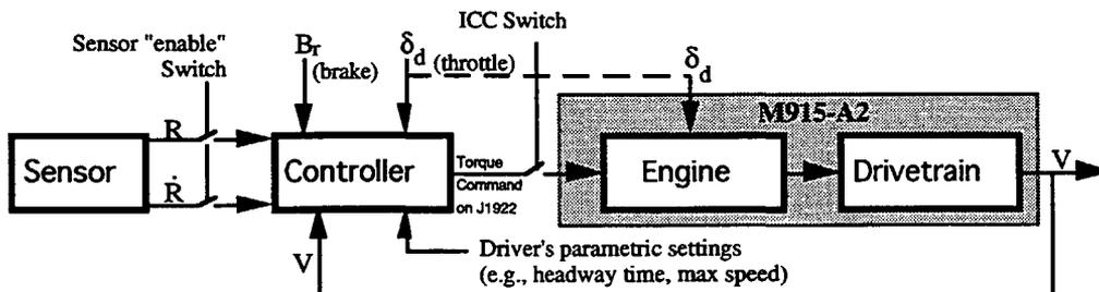
Figure 5. Control setup as implemented in the testbed
