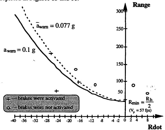
Figure 15. Deceleration boundary that calls for driver's intervention,  $T_h=1.5$  sec.
