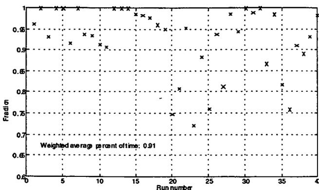
Figure 11. Fraction of time range rate was  $\pm 1$ fps during following
