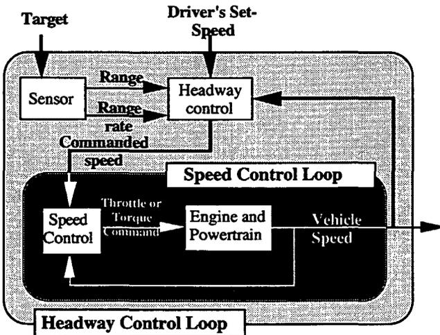
Figure 4. Headway control and speed control loops used in intelligent cruise control
