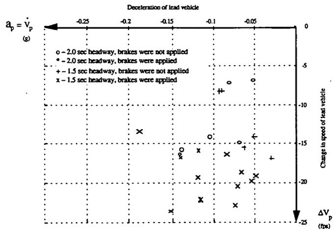
Figure 13. Braking results for speed changes by the lead vehicle
