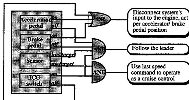
Figure 6. System's logic and control inputs
