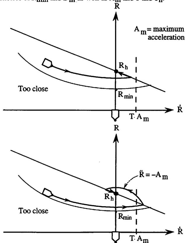
Figure 10. Sudden target acquisition
