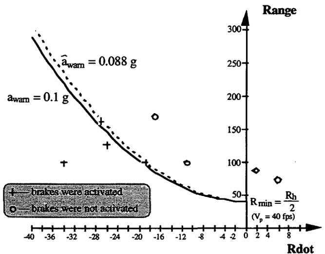
Figure 16. Deceleration boundary that calls for driver's intervention,  $T_h=2.0$  sec.
