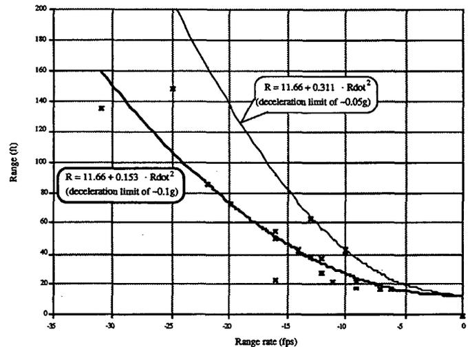
Figure 17. Brake activation points
