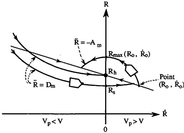
Figure 3. Parabolic trajectories of constant acceleration
