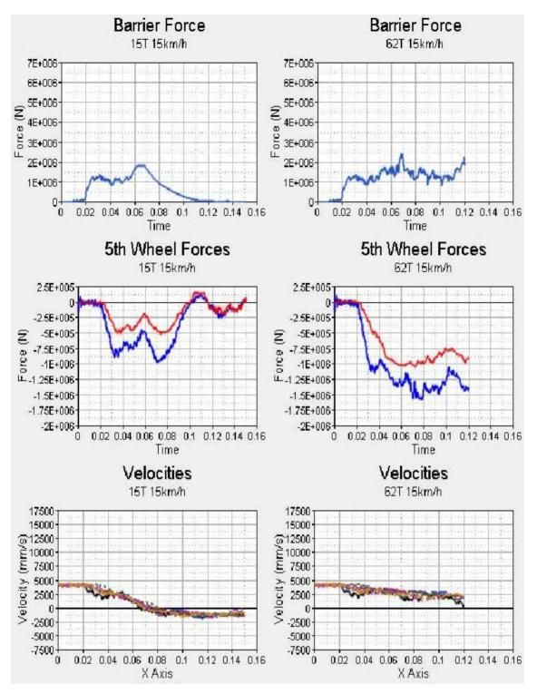
Figure 8a Force and velocity results for 15 km/h impacts.
