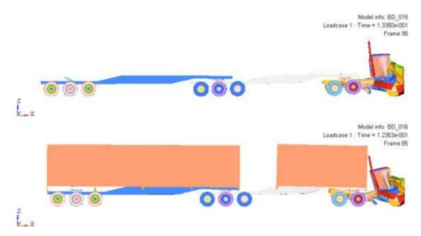
**Figure 6** A pictorial representation of the crash damage to the B-double (60 km/h).
