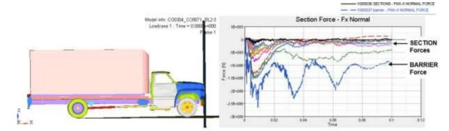
Figure 3a Force results for the barrier crash
