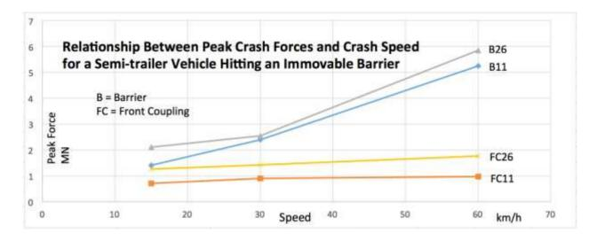
Figure 9 Peak force for both masses plotted against initial speed; for the B-double truck.
