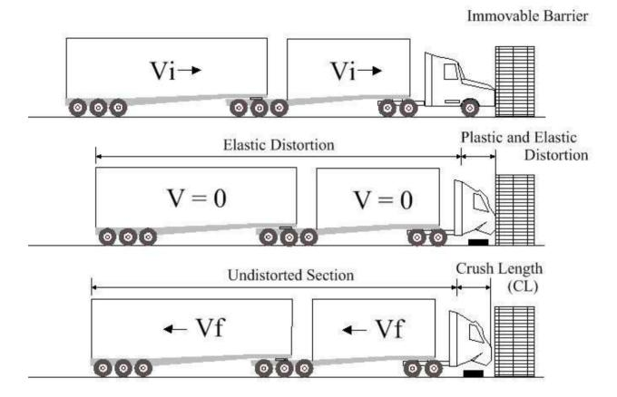
Figure 3 Simplistic representation of plastic and elastic sections of the crash vehicle.
