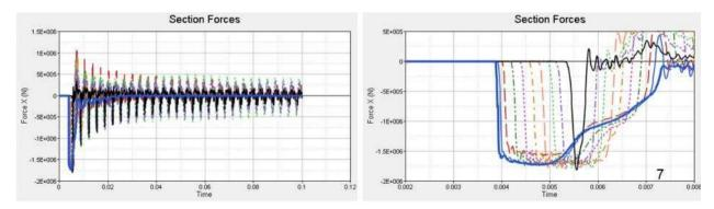
Figure 4Shock waves in the chassis-rail ladder of the rigid truck
