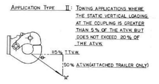
**Figure 10** The proof-test specification that is in SAE J847.
