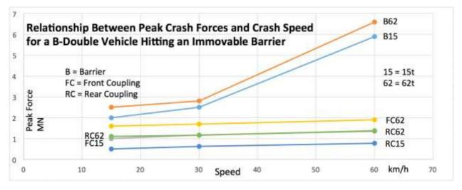
Figure 7 Peak force for both masses plotted against initial speed; for the B-double truck.
