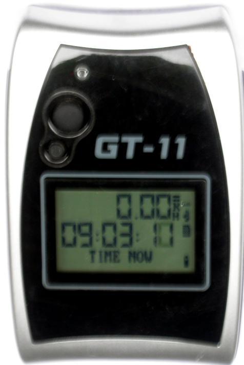
**Figure 5** - The GPS-11 data recorder. The display shows real time and instantaneous speed.
