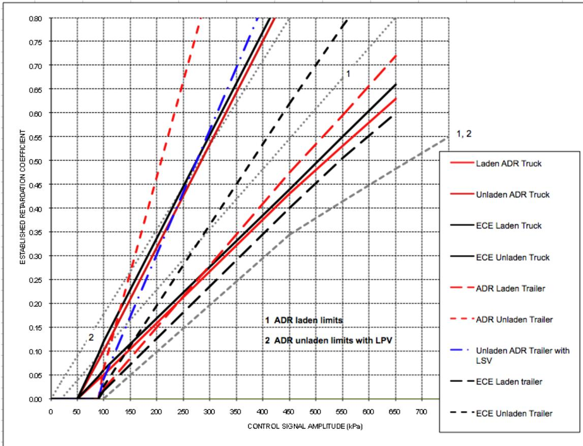
**Figure 5** The nominal vehicle set-ups. The tests were conducted with control pressures in the range 160 – 390 kPa.
