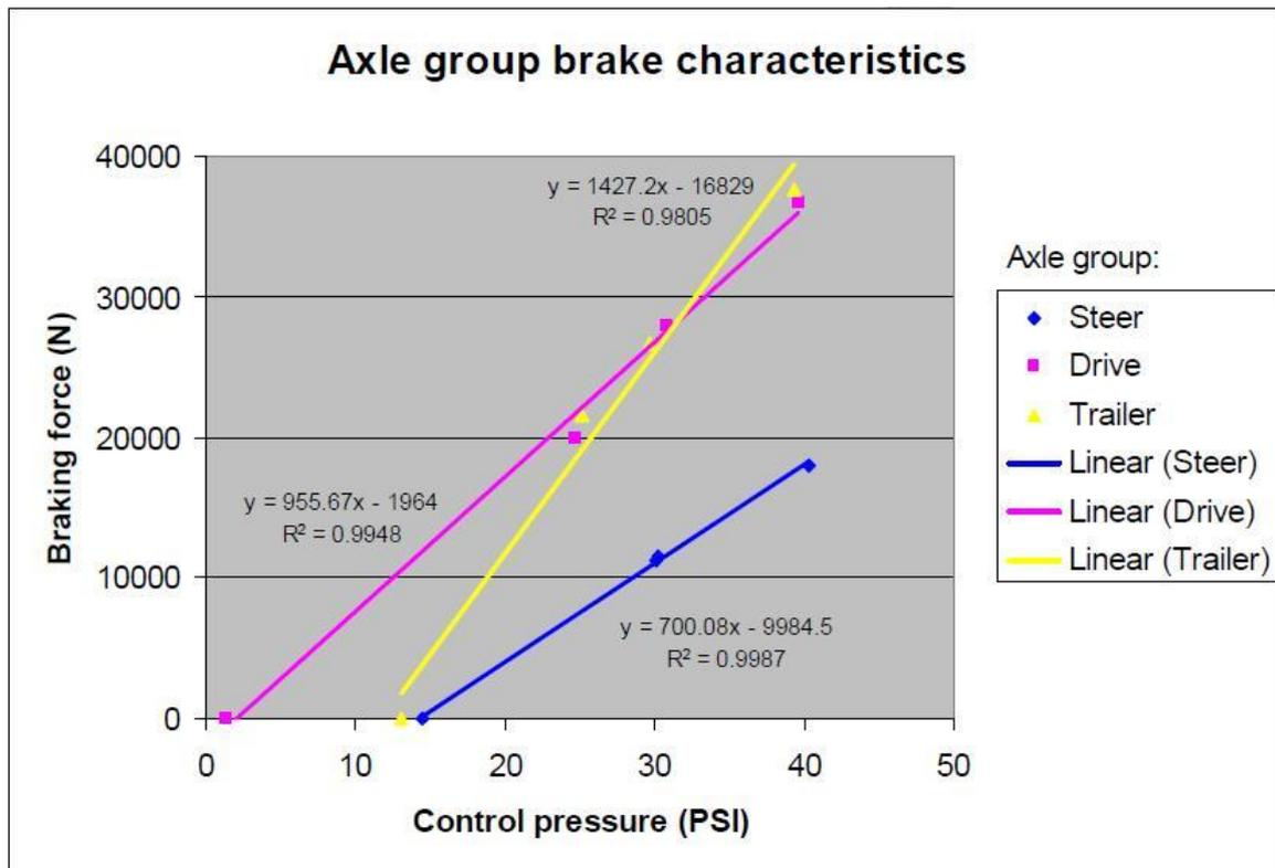
**Figure 4** Axle-group force characteristics.
