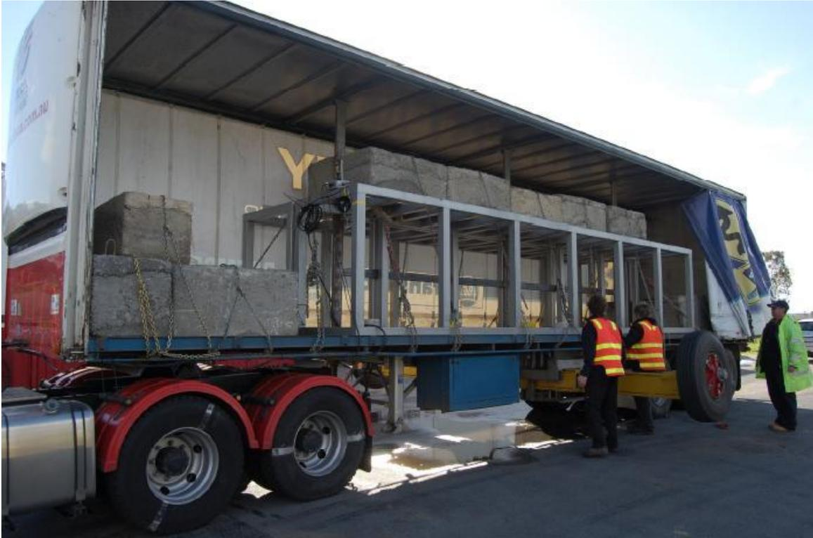
**Figure 3** The load at the front of the trailer was at floor level. A 1.5 m high load frame was used to increase the height of the load towards the rear.
