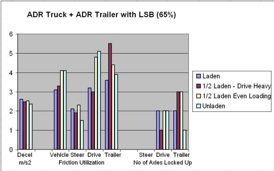
**Figure 7** ADR truck & ADR trailer with an LPV set to 65% (unladen).
