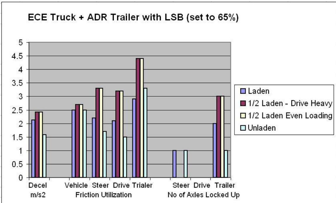
**Figure 11** ECE truck & ADR trailer with LSV set to 65%.
