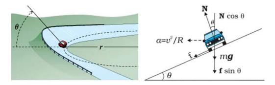
Figure 2 - Basic analysis of cornering forces [Mastering Physics & Physics365.com]
