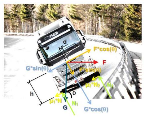
Figure 4 - More accurate analysis of cornering forces in heavy vehicles
