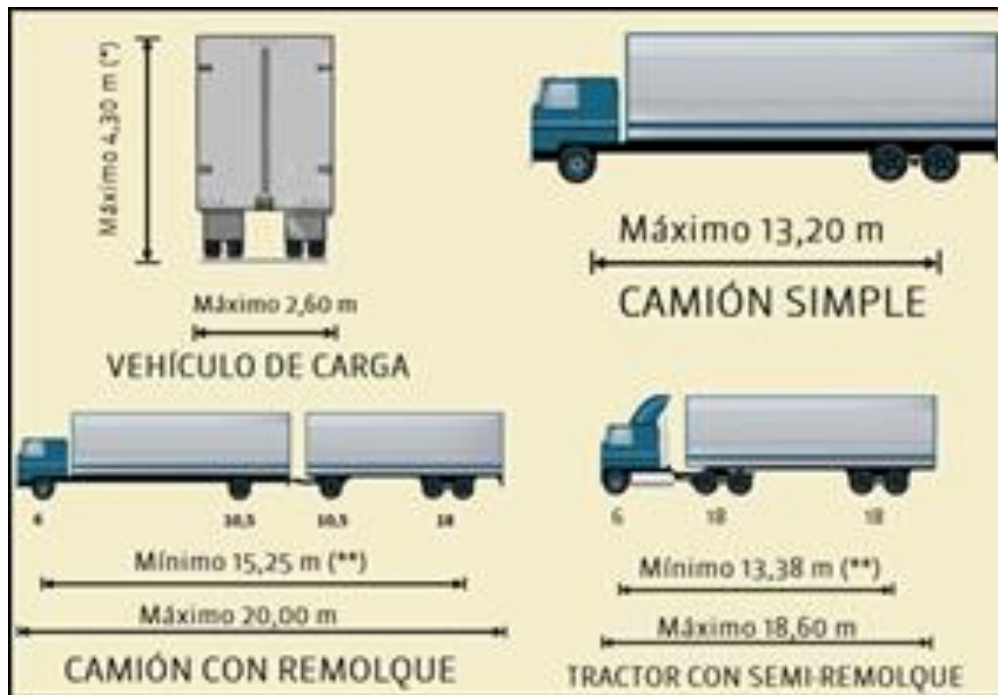
Figure 1 - Types of vehicles that consume 75% of equivalent axles, measured in weight stations (left), and type of authorised heavy vehicles in Uruguay (right)
