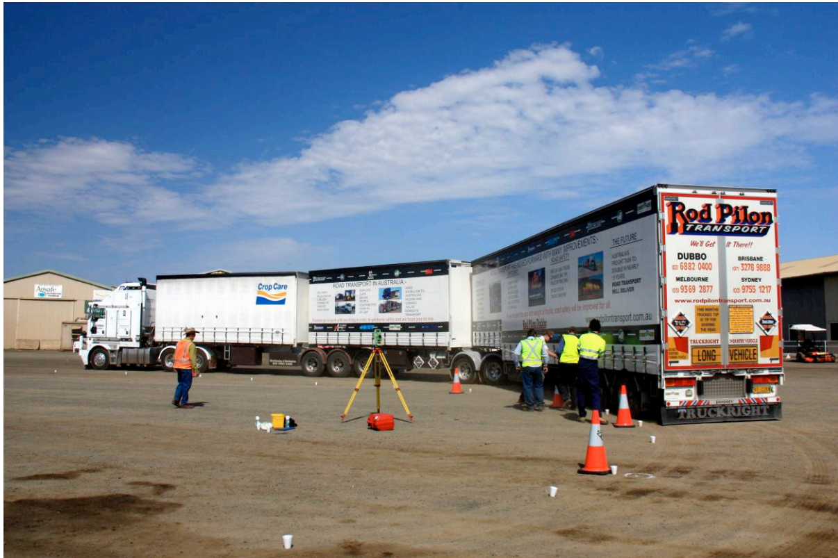
Figure 6 – On-road testing of B-triple vehicle
