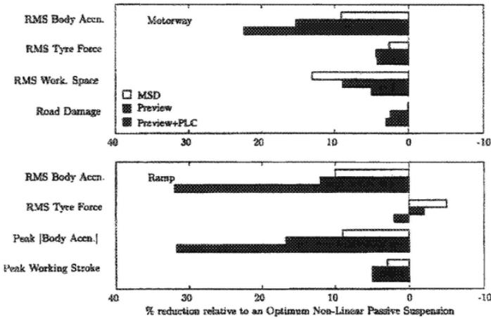
Figure 5: Summary of the measurements with the prototype semi-active damper using a four DOF HiL test rig. All criteria with the exception of road damage relate to the measurements at the drive axle only. (a) Motorway; (b) Filtered step (ramp).
