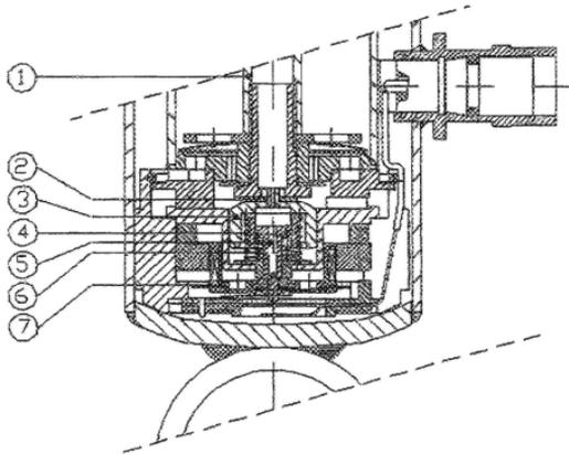
Figure 6: Diagram showing sectioned view of base of damper.
