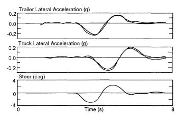
Figure 7/ Comparison Between Test and Simulation Truck-Pony Trailer, Short Hitch Offset, 60 km/h
