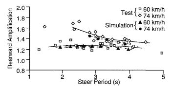
Figure 8/ Truck-pony Trailer Stability Analysis, Nominal and 4-foot Hitch Offset
