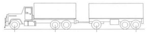
Figure 4. Three-axle truck and three-axle dog trailer.
