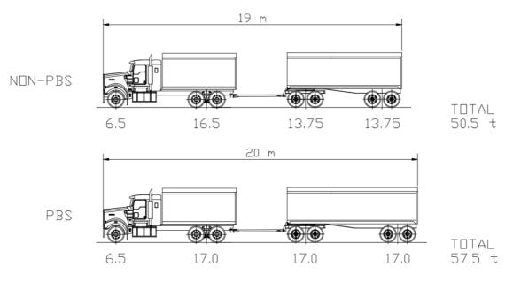
Figure 3 – Difference between non-PBS and PBS truck and dog
