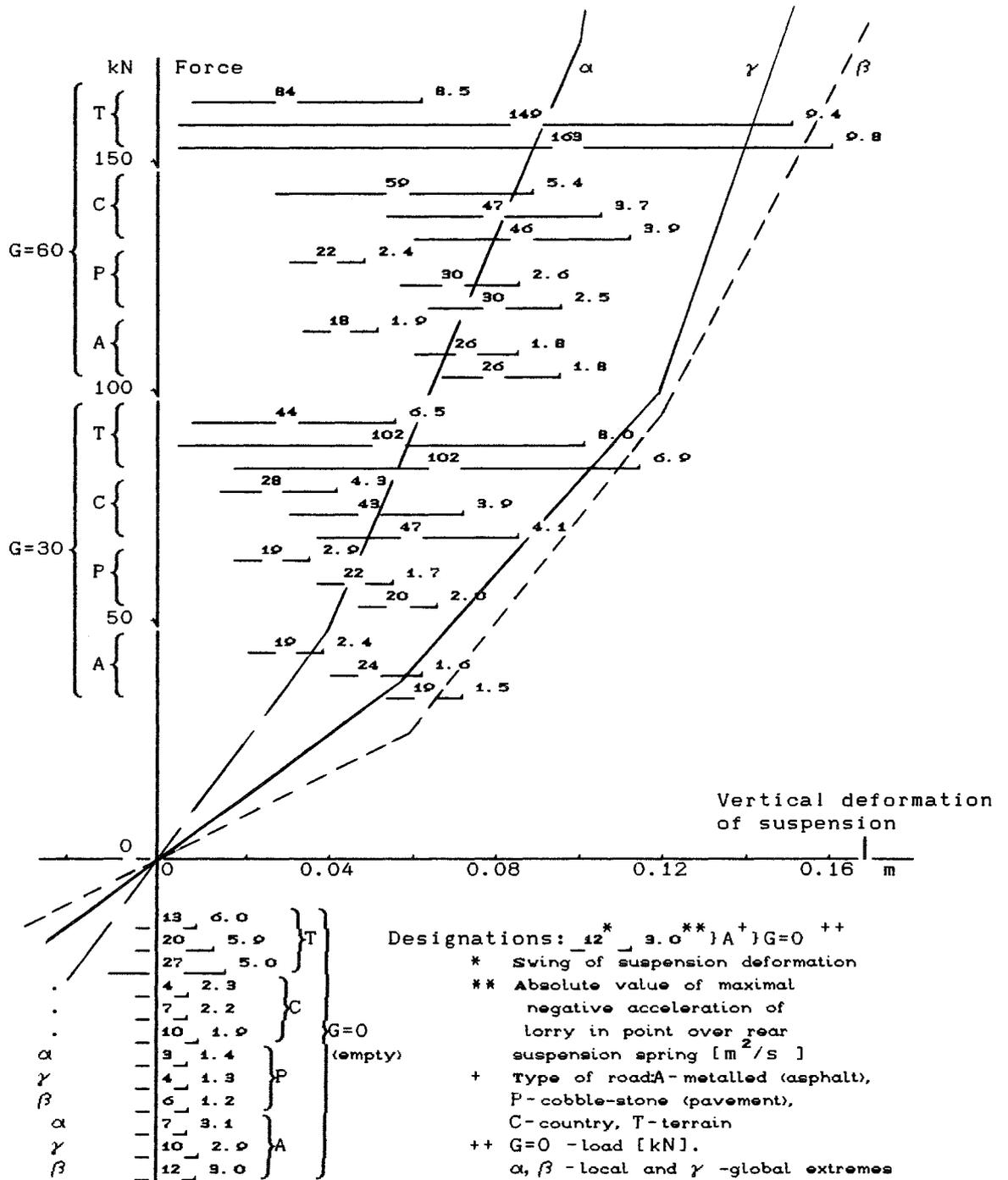
Fig. 3. Schematic diagram of suspension spring force
