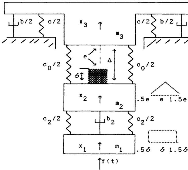
Fig. 4. Dynamical scheme of a crumbling machine
