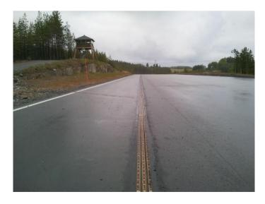
Figure 4 - The Elways electric beam on a test site.
