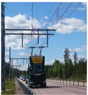
Figure 3 - The Siemens e-Highway system demonstrated outside Sandviken in Sweden.
