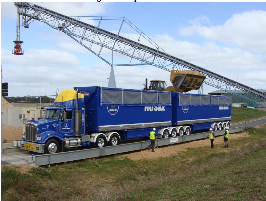
Figure 7 – Super B- double – Loading. Please note it is resting on weighing scales
