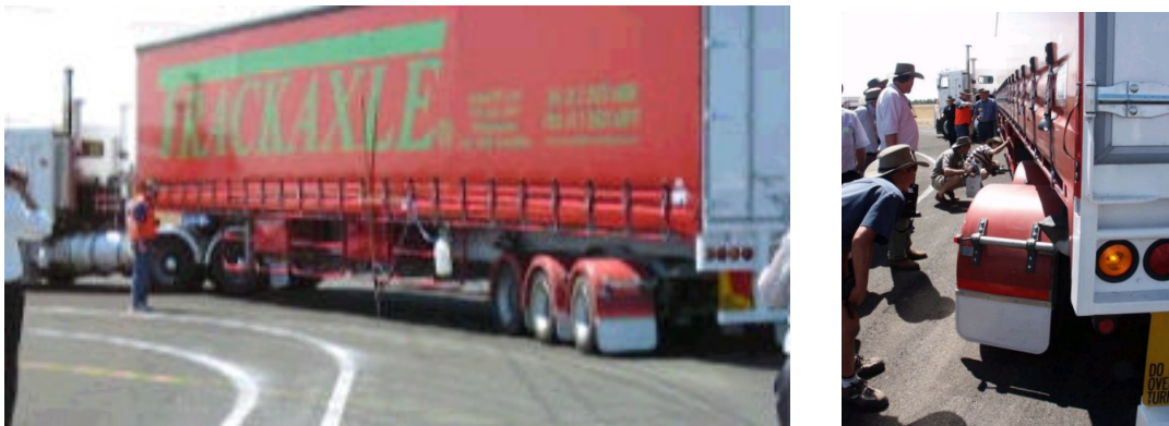
Fig. 2 - Trackaxle® demonstrator performing a low-speed turn at the PBS International Seminar (National Transport Commission, 2003).
