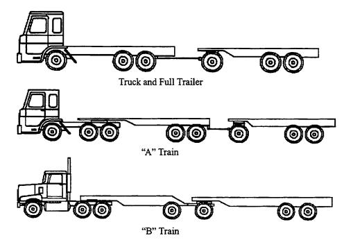
Figure I: New Zealand vehicle configurations
