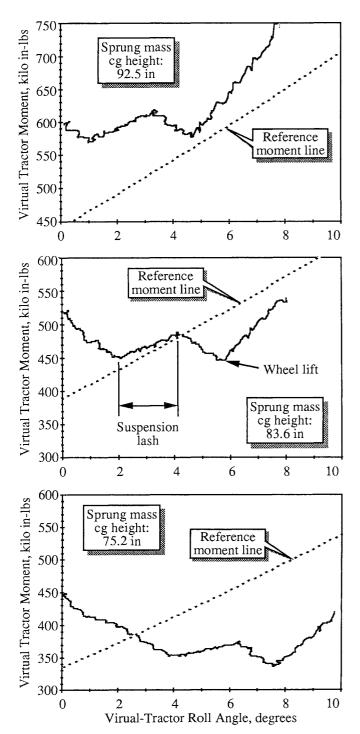
Figure 8. Tilt-table data from tests of a semitrailer with three different cg heights
