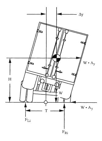
Figure 1. A heavy truck in a steady turn
