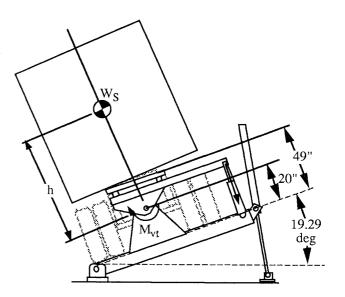
Figure 2. A tilt test using the virtual trailer
