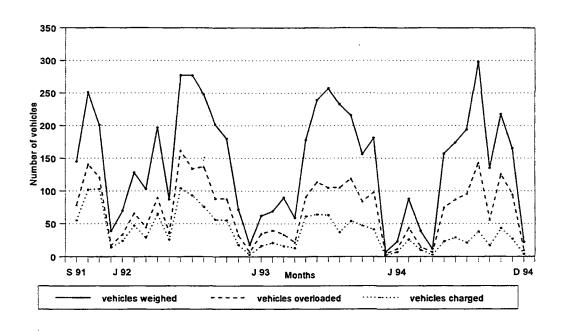
Figure 6. Vehicles weighed, overloaded and charged per month of UNITRANS: September 1991 to December 1994
