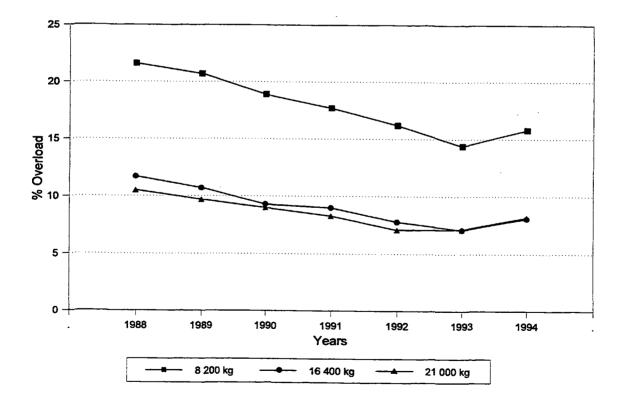
Figure 4. Average overloads in KwaZulu-Natal: Single axles, tandems and tridems: 1988 to 1994
