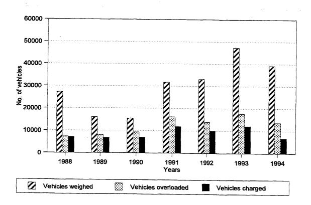
Figure 2. Vehicles weighed, overloaded and charged per year in KwaZulu-Natal: 1988 to 1994
