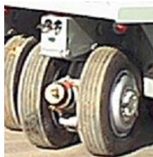
Figure 1 – Early example of an SWS steerable wheel group.
