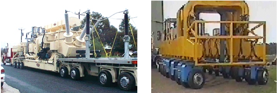
Figure 3 – Two example demonstrators showcasing SWS wheel group technology; a platform trailer (left image) used to transport indivisible loads (a transformer shown) and a straddle carrier (right image) for transport of metal ingots.
