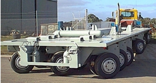
Figure 2 – Early application of the SWS steerable wheel group in a multiple wheel-group (3 per “axle”), multiple-row (6 axles) load platform.
