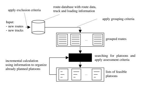
Figure 3 – Illustration of Our New Algorithm to Find Truck Platoon Sequential Pattern
