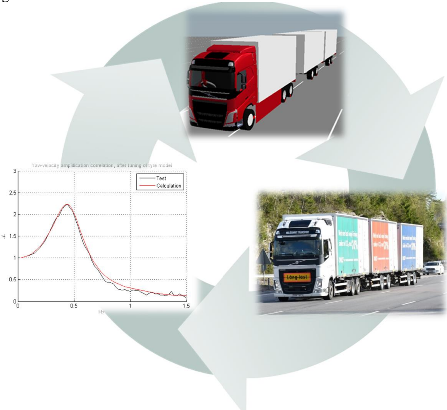
Figure 5 – correlation of complete vehicle performance by tuning the trailer tires cornering coefficient and relaxation.
