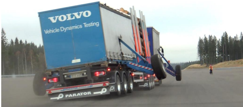
Figure 11 – lift of the last wheels on a B-double, but the load transfer ratio is not 100%
